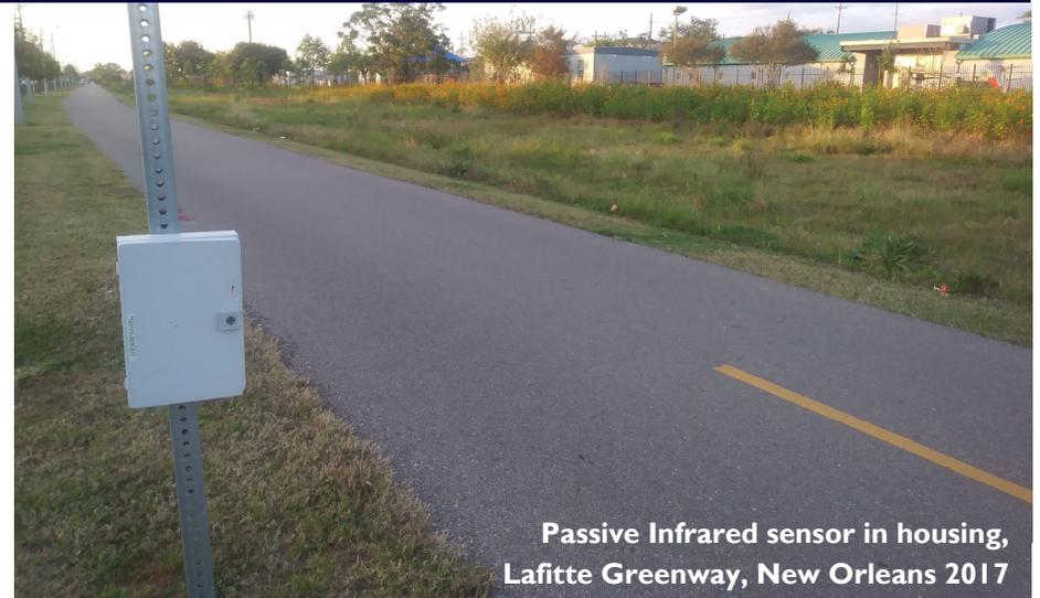
Passive Infrared sensor in housing,
